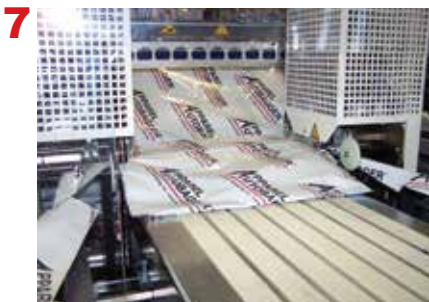
7 Dimensions are scanned and package is wrapped and sealed to form mailer.
