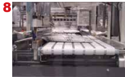
8 Adapta feature forms right-size package for reduced DIM and shipping cost.
