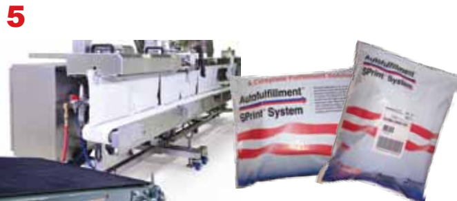
Seal flattener ensures a wrinkle-free, secure seal.
