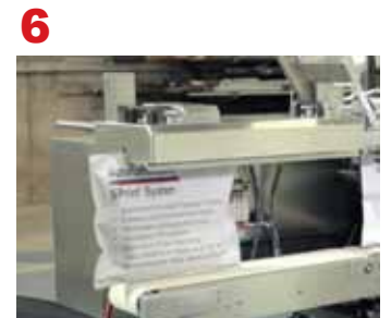
Mailer is sealed with 3/8" heat seal and then exits the system.
