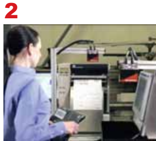
Packslip prints and drops into mailer automatically.
