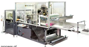
The Accutech Returns Processing System automates the process of polywrapping returned merchandise so that it is suitable for going "back to stock."
