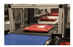
The Apparel Autobagger operates by transporting product on a belt between two rolls of film - top and bottom. The mailing label is printed on the top film and then the top and bottom are sealed together surrounding the product. The mailers will be right-sized in both directions.
