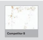
**Fiber Pull Demonstration:** Shows how much paper fiber the tape pulls off the recycled corrugate box upon removal. The higher percent of fiber pull, the stronger the tape bond is to the box.
